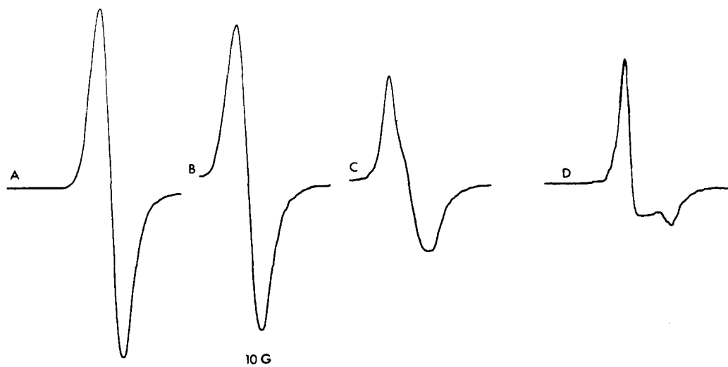
Fig. 2. Electron spin resonance time-profile of daunomycin (1 mg/ml) in the presence of GSH (10-fold excess), microsomes (1.5 mg/ml protein), and NADPH regenerating system under anaerobic conditions. The nominal microwave power was 20 mW and the modulation amplitude was 0.6 G. A: 2.0 min (receiver gain 4 \times 10^3 ); B: 10 min (receiver gain 8 \times 10^3 ); C: 3 min (receiver gain 8 \times 10^3 ); and D: 2.0 hr (receiver gain 1.6 \times 10^4 ).
